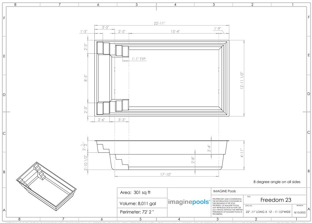
**NOTE:** THE MEASUREMENTS ON THIS DIG SCHEMATIC ARE PROVIDED ONLY AS A REFERENCE AS THE EXCAVATION NEEDS FOR EACH INSTALLATION MAY VARY. IN ADDITION, FROM TIME TO TIME WE MAY MAKE ENHANCEMENTS TO THE POOL LAMINATE CONSTRUCTION WHICH IN SOME CASES MAY RESULT IN MINOR ALTERATIONS TO THE MEASUREMENTS PROVIDED. PLEASE ENSURE THAT YOU ARE USING THE MOST CURRENT SCHEMATIC AS A REFERENCE FOR YOUR INSTALL AND INSPECTING THE INDIVIDUAL POOL FOR ANY NECESSARY ADJUSTMENTS.
