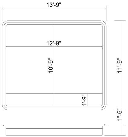
(Add approx 1" for fiberglass floor thickness)
